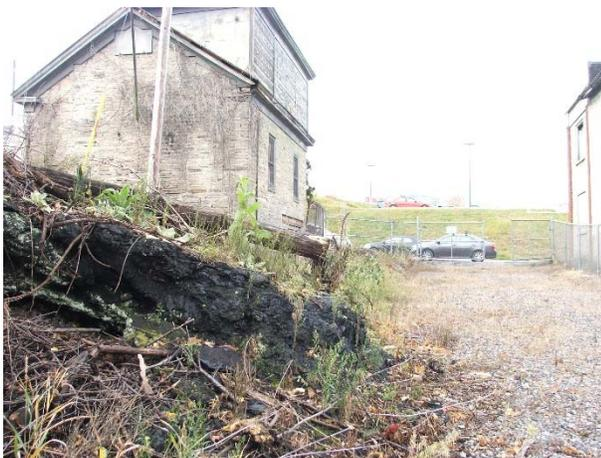
Figure 3-2 Solid tar observed on ground surface of site, looking toward Amsden Street, former MGP building on left
