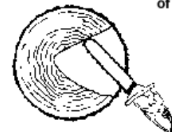
Top or blade nose touches bottom or side of kerf during reinsertion
