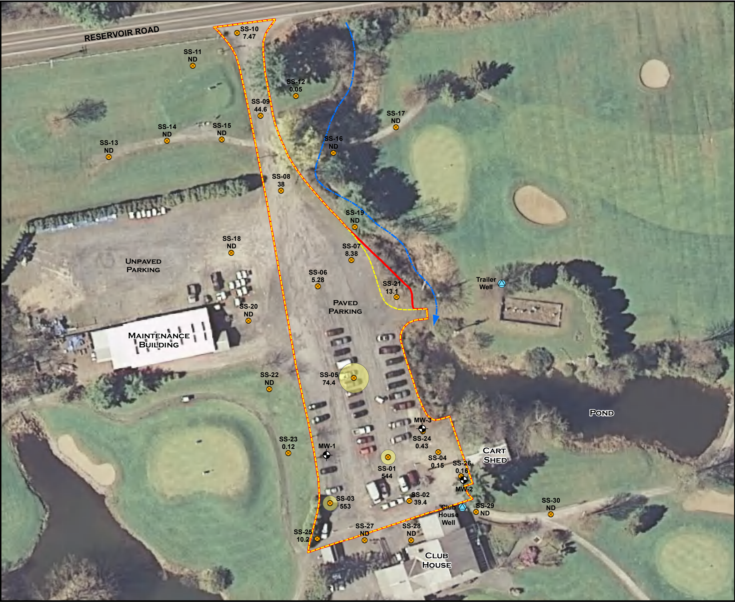
FIGURE 4 REMEDIAL ALTERNATIVE 3 EXCAVATION OF SOILS W/PCBs \geq 50 PPM & INSTALLATION OF ASPHALT PAVING CAP
