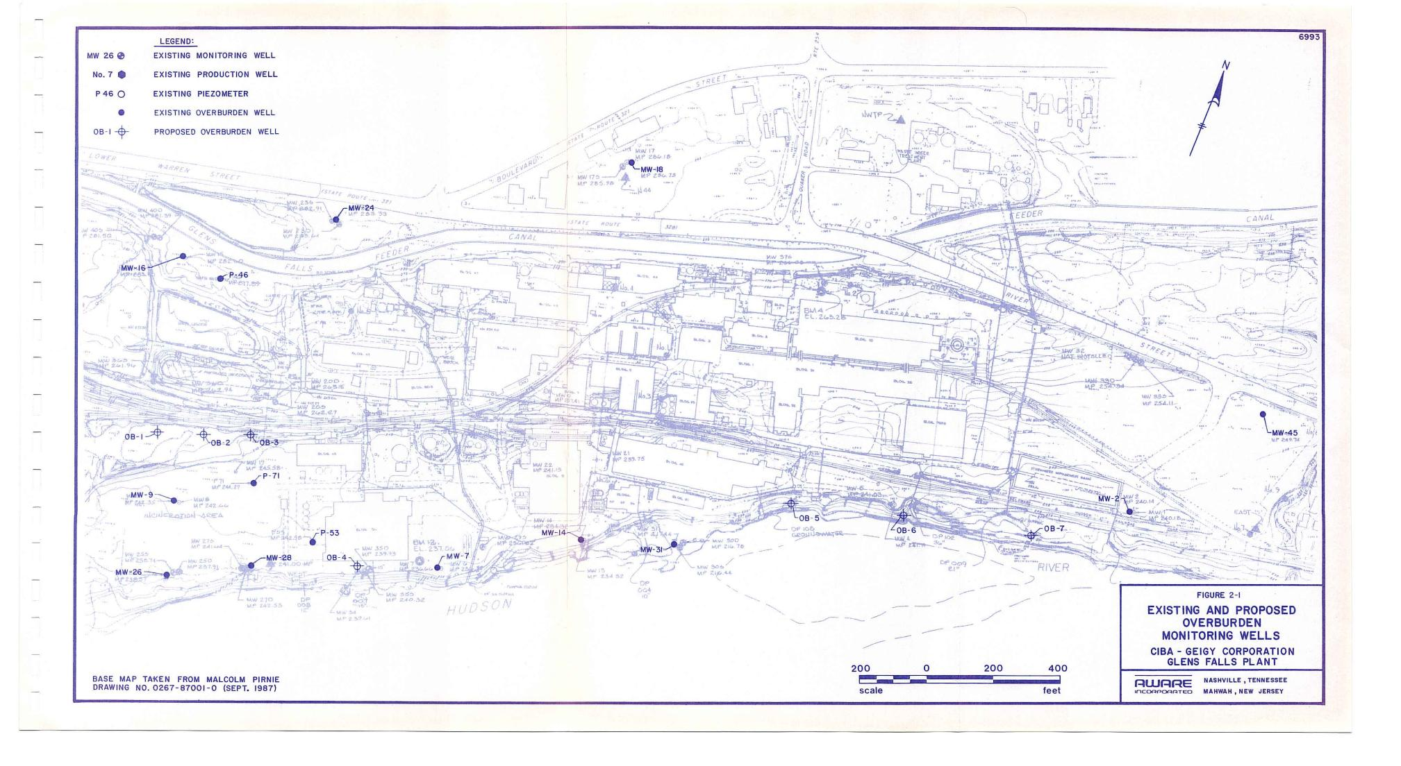
(1986) and under the general oversight of NYSDEC. Wells with an open interval from approximately five to fifteen feet below top of rock were identified as shallow ("S") and wells open from 25 to 35 feet below top of rock were identified as deep ("D").
