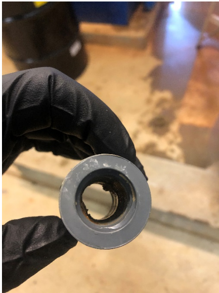
View of fracture and buildup inside Bleach PVC coupling.
