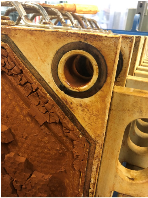
View of cracked Filter Press O-ring.
