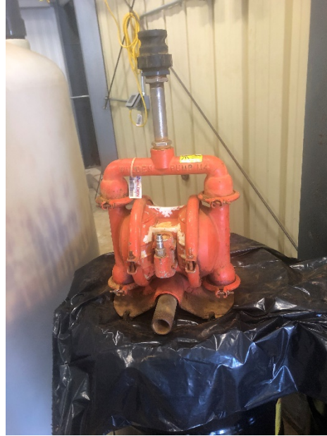
Replaced diaphragm on spare feed pump.
