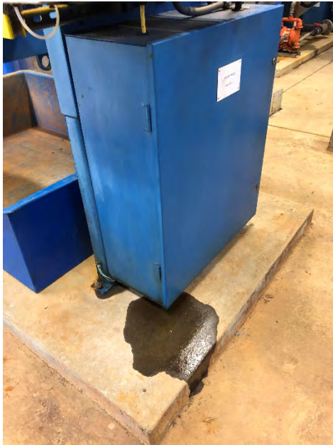
View of Filter Press hydraulic leak prior to repairs.
