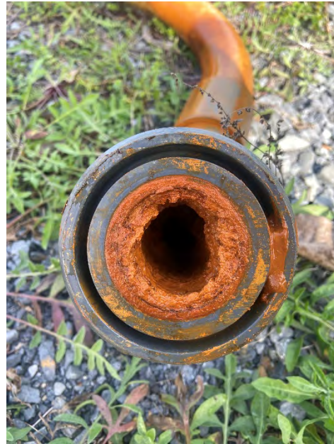
View of scaling within EW-4 secondary manhole piping.
