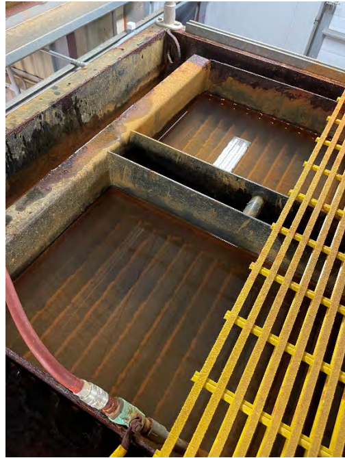
View of IPC plates prior to spray down.
