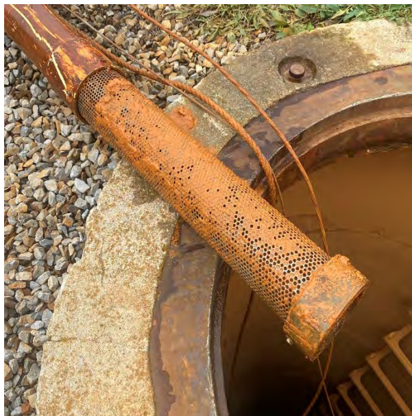
View of EW-4 pump screen after one week of use.
