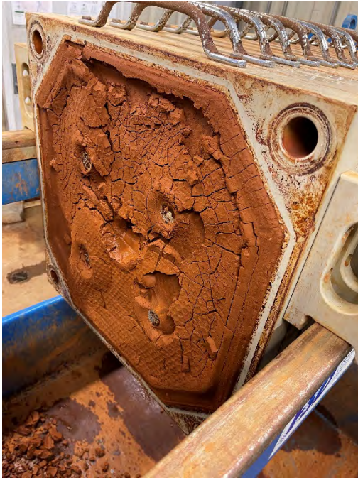
View of Filter Press sludge following cake discharge.
