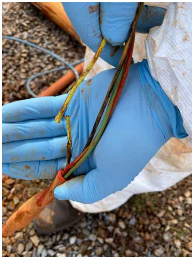
View of damaged wire on EW-4 pump.
