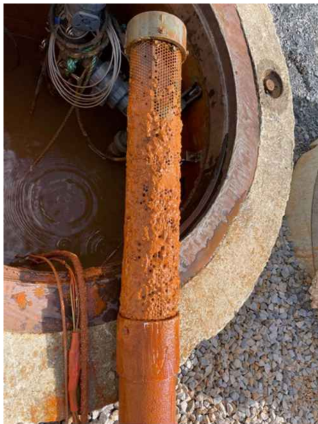
View of clogged EW-4 pump screen.
