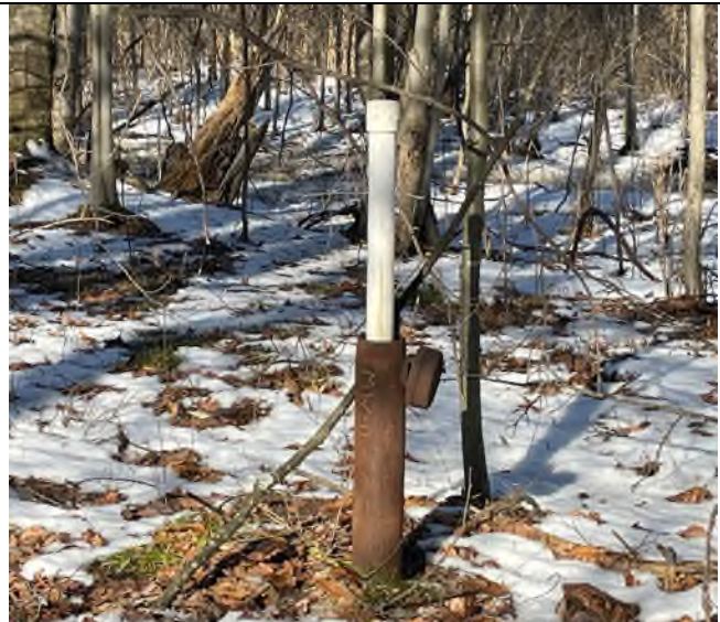
Monitoring well MW-11 with previously identified protruding well riser.
