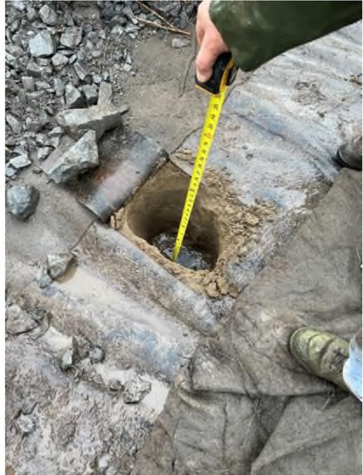
8. Cap Liner Found at 12" below swale – Test Pit #2B.
