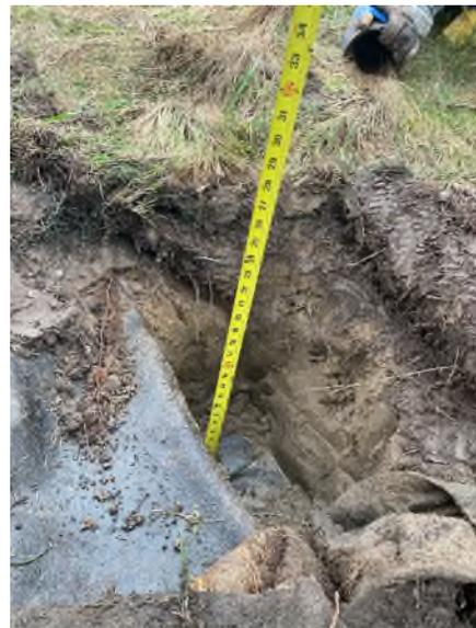
10. Cap Liner Found at 14" below edge of swale at Test Pit #2C.
