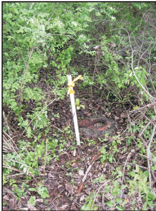
Photo 10: Piezometer PZ-3. PVC pipe placed in ground to help locate flush mount well in the future.
