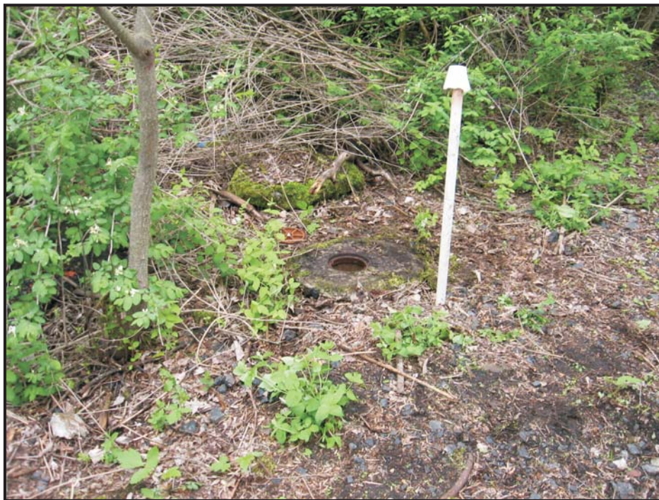
Photo 11: Piezometer PZ-4. PVC pipe placed in ground to help locate flush mount well in the future.
