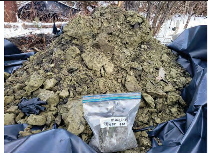
Photo 8: Soils recovered from the TP-102 test pit excavation, from the 2 – 4-foot interval. Facing north.
