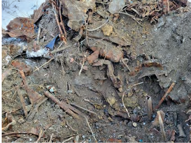
Photo 61: Sidewalls at the TP-116 location, which contains a large percentage of percentage of scrap metal and miscellaneous wastes, facing south.
