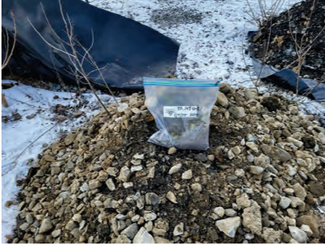
Photo 33: Soil recovered from the TP-108 excavation from the 0 – 2-foot interval, facing west.
