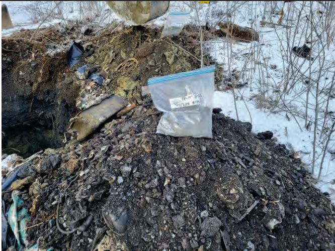
Photo 35: Soil recovered from the TP-109 location from the 0 – 2-foot interval, note the scrap metal/wires/ash/plastics present. Facing north
