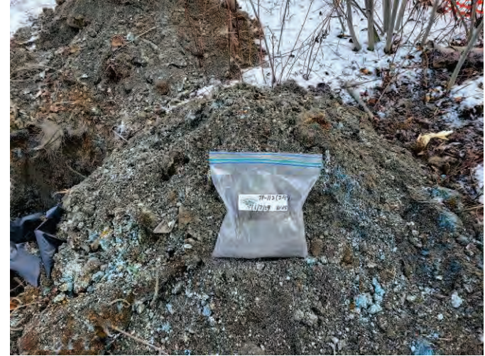
Photo 46: Soil/ash recovered from the TP-112 test pit excavation at the 2 – 4-foot interval. Facing south.
