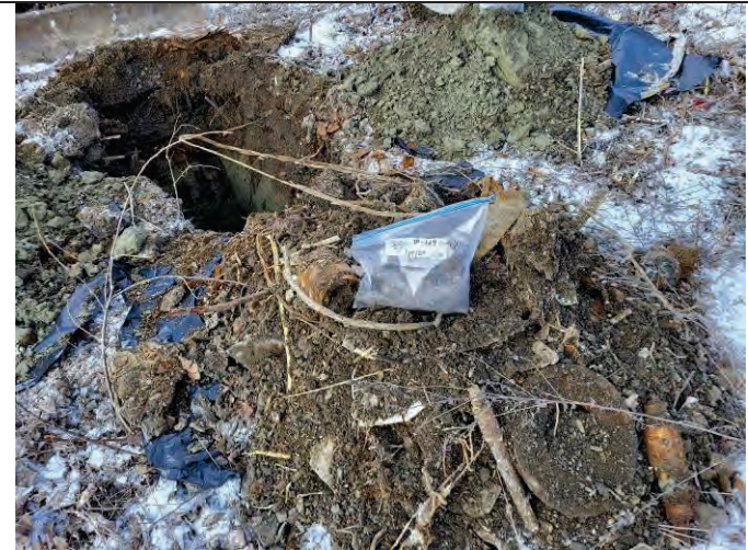
Photo 16: Soil recovered from the TP-104 borehole from the 0 – 2-foot interval. Note the presence of scrap metal, wires, plastics and ash. Facing north.
