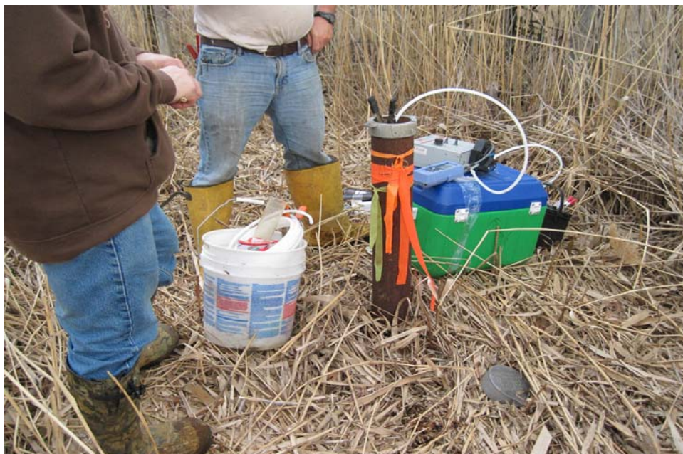
Photo 14: Low flow sampling setup at MW-4.
