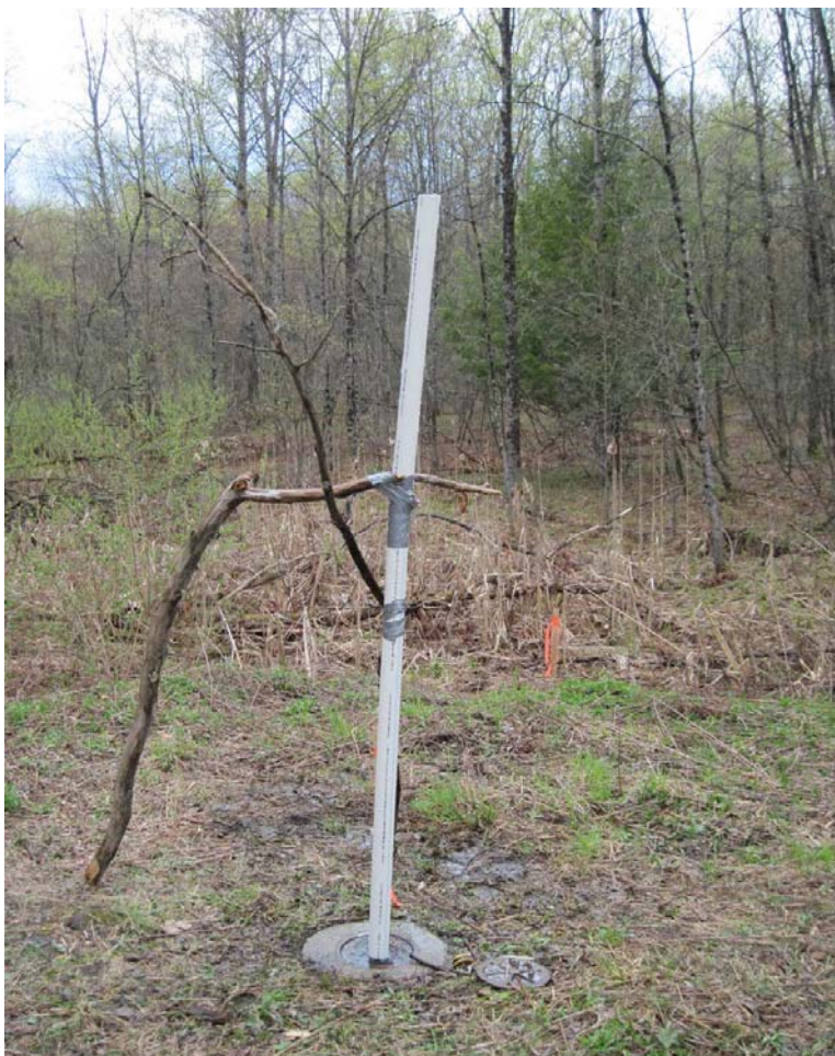
Photo 13: Additional PVC riser added to SW-04D in an attempt to obtain a water level due to the artesian conditions of the well.
