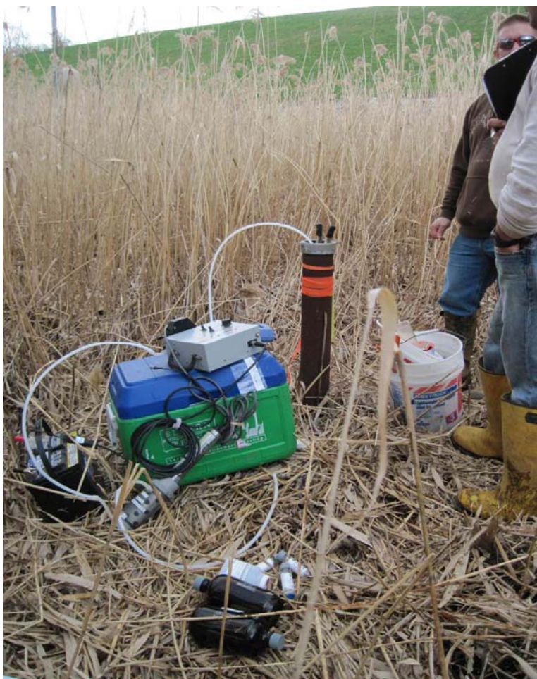
Photo 15: Low flow sampling setup at MW-3.
