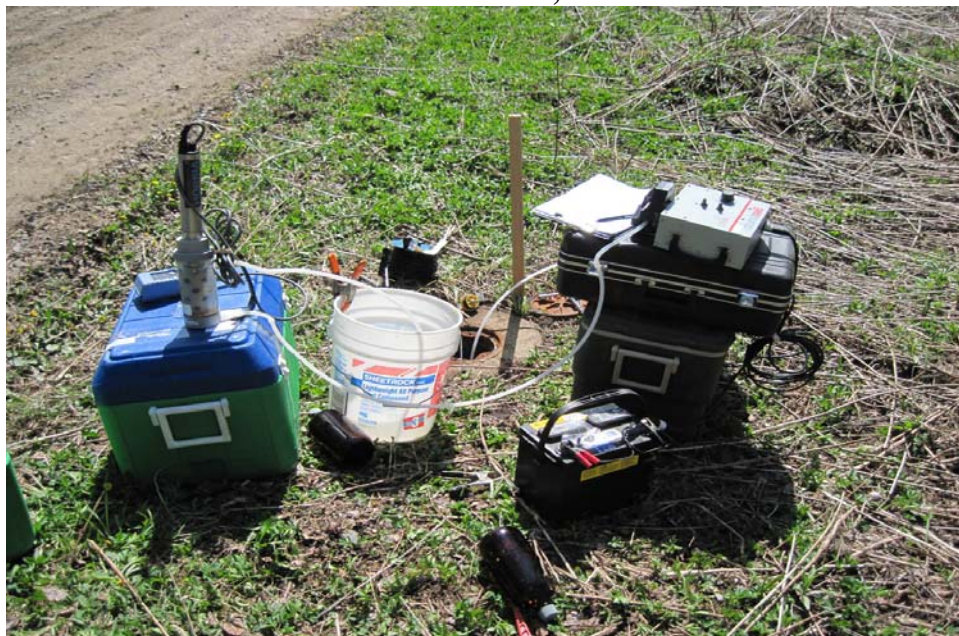
Photo 12: Low flow sampling setup at SW-04S.
