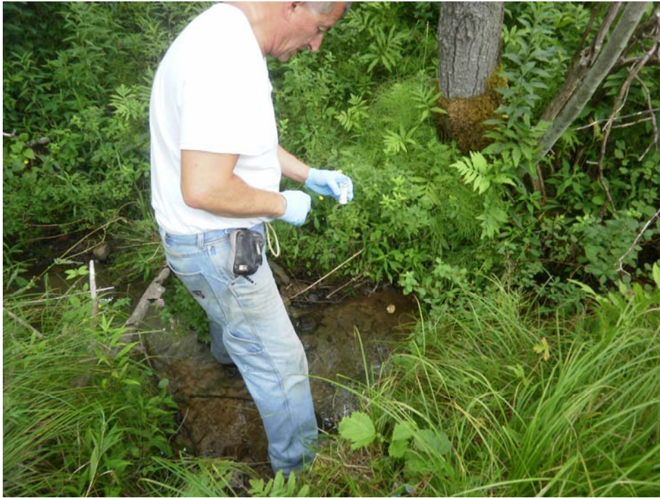
Photo 9: 7/11/2011-Collection of surface water sample from location SWTR-1E.
