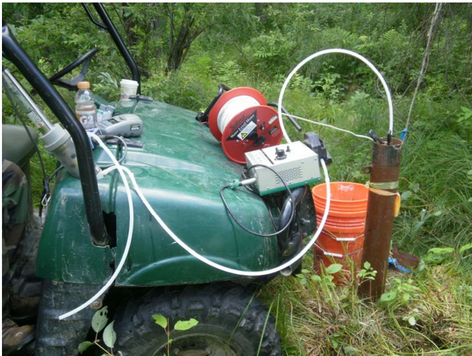
Photo 10: 7/11/2011-Low flow sampling setup MW-16 in the background.
