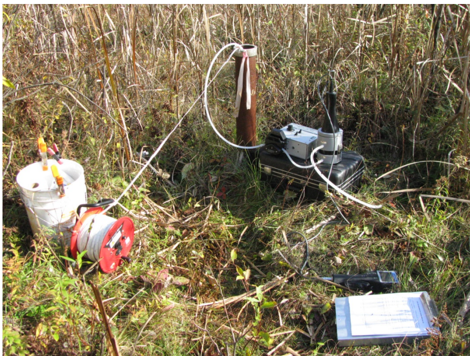
Photo 28: 10/18/12 Typical low-flow groundwater sampling set-up. Photo taken at location MW-04.
