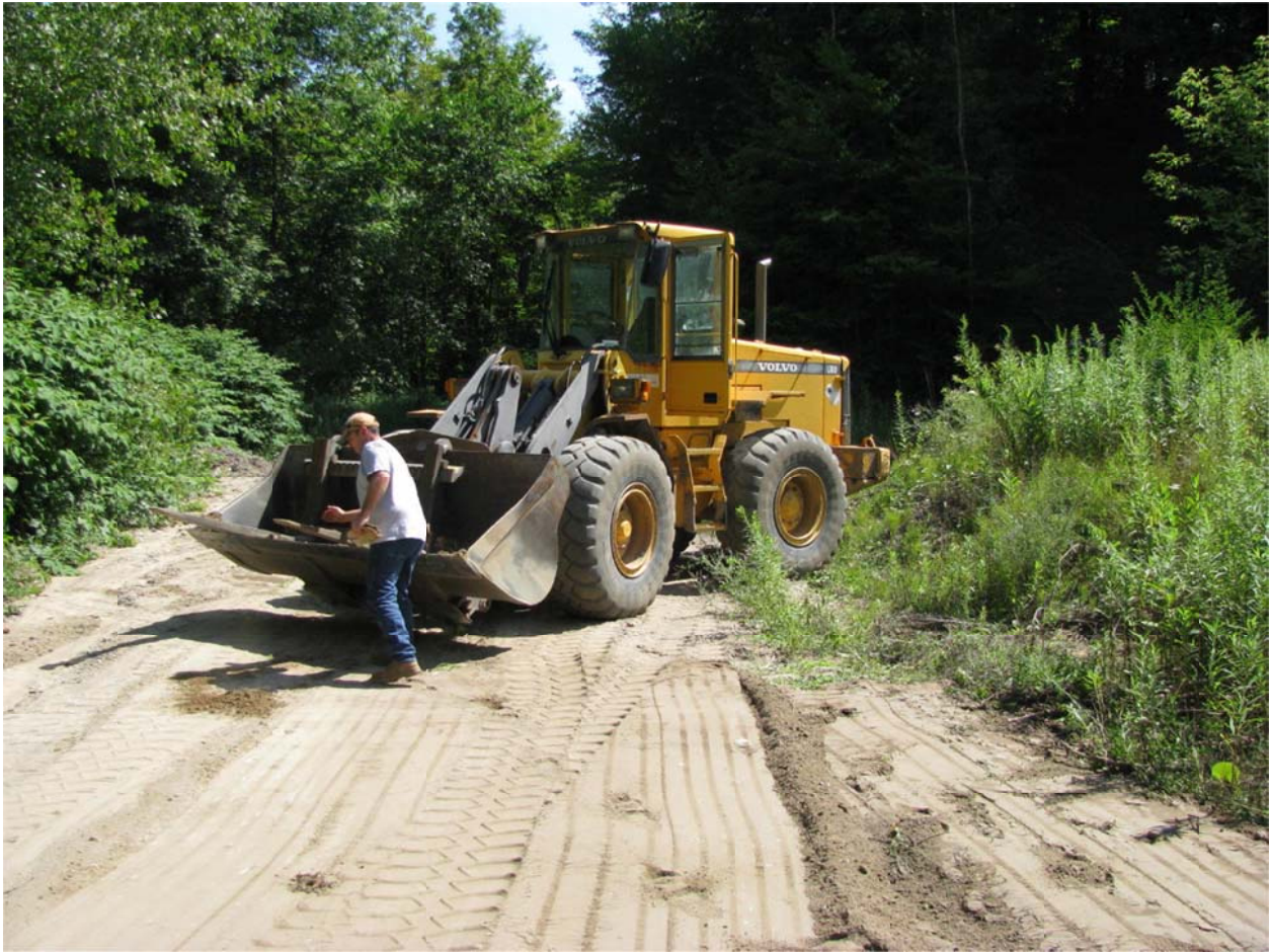
PHOTO 2: Excavator used to position jersey barriers. Note fork attachment in bucket.
