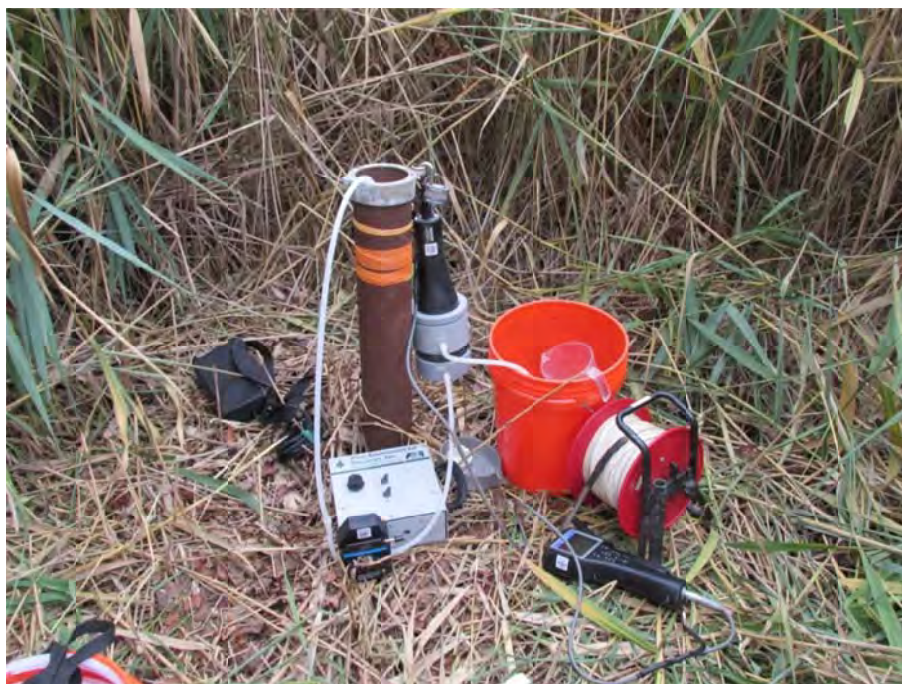
Photo 26: 10/16/13 Typical low-flow groundwater sampling set-up. Photo taken at location MW-03.
