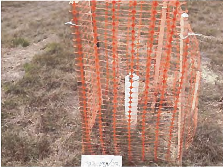
5. Monitoring Well Protective Measure Example
