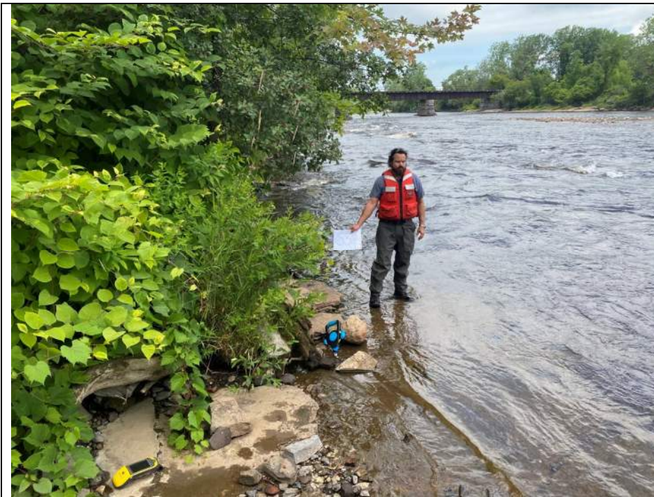
Photograph #1 (7/12/22) – Area of S3 deposit. View looking downstream (northwest). Hardened tar visible in root structure of fallen tree and faint tar odor when disturbed.
