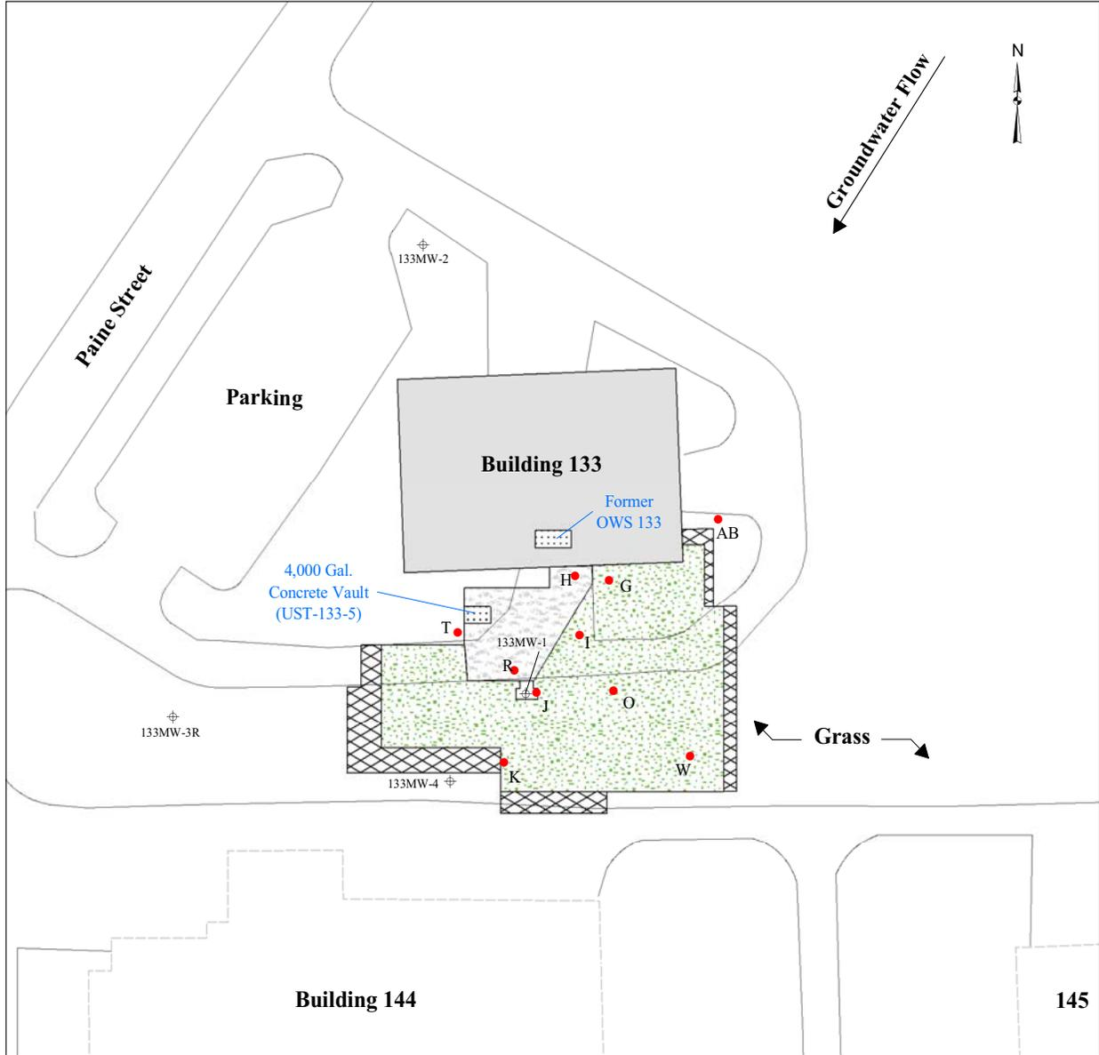
**Figure 3 : Building 133 Excavation & Overexcavation Extents**
