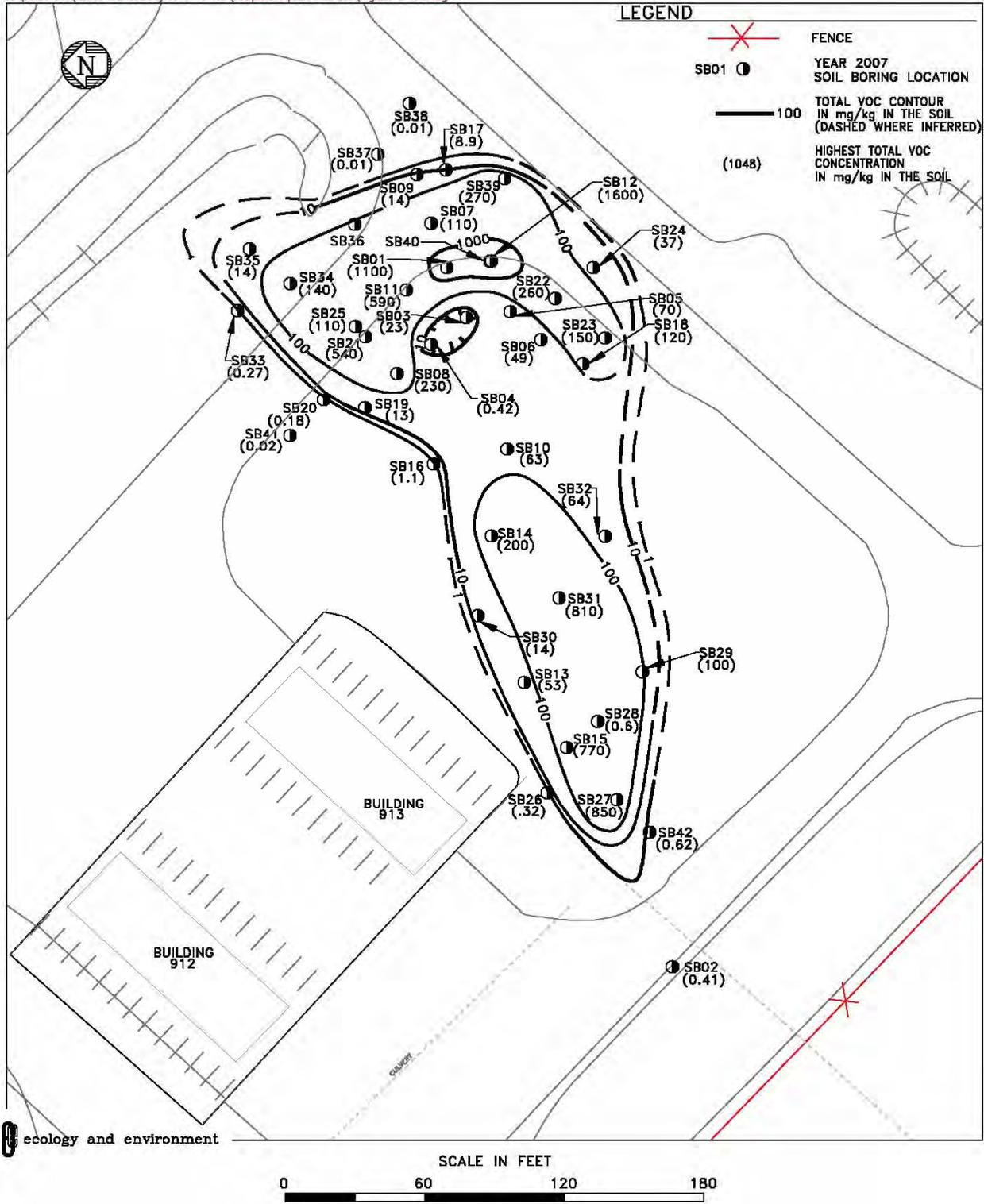
Figure 5 Soil Boring Locations and Total VOC Contours
