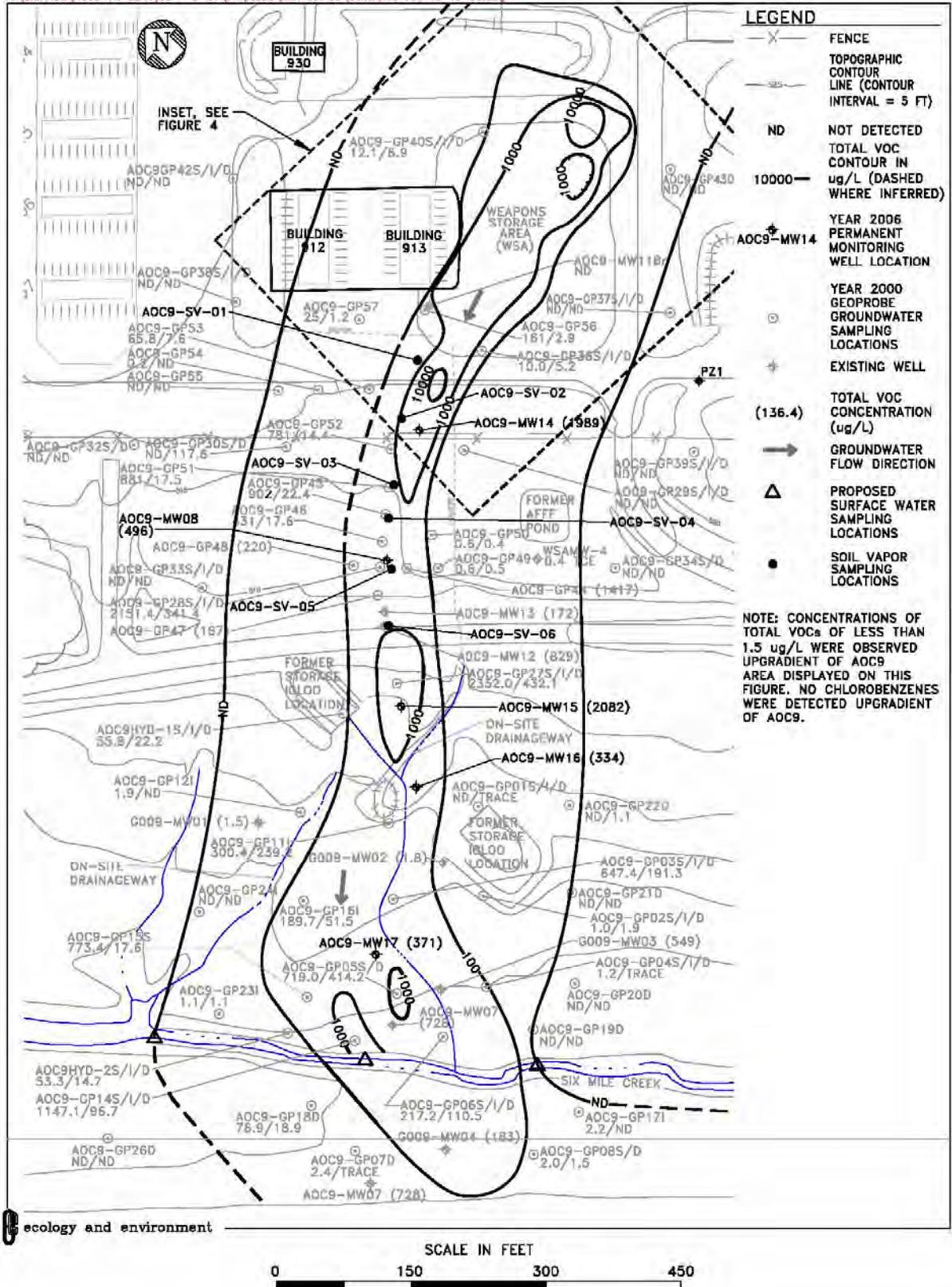
Figure 3 Total VOC Concentrations in Groundwater and Soil Vapor Sample Locations
