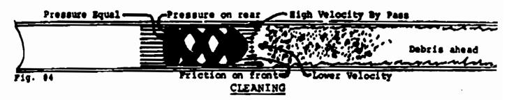
When a Girard Polly Pig is run through the line the following takes place: (A) Frict drag on the front (B) Pressure applied to the rear (C) These two forces meet in the middle making the pig shorter and directing the forces to the outside (D) A high velby-pass from rear to front past the pig resulting in a sliding seal thus helping to loose deposits and flushing ahead of the pig.
