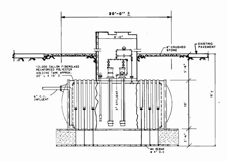
NOTE: INFLUENT AND EFFLUENT PIPING SEALED-OFF DURING UST ABANDONMENT IN 1987
