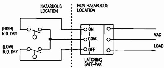
Latching SAFE-PAK, Part Number 41705 or 41715 handling high and low level sensors located in hazardous area for pump-down control. For pump-up, use two N.C. dry switches.
