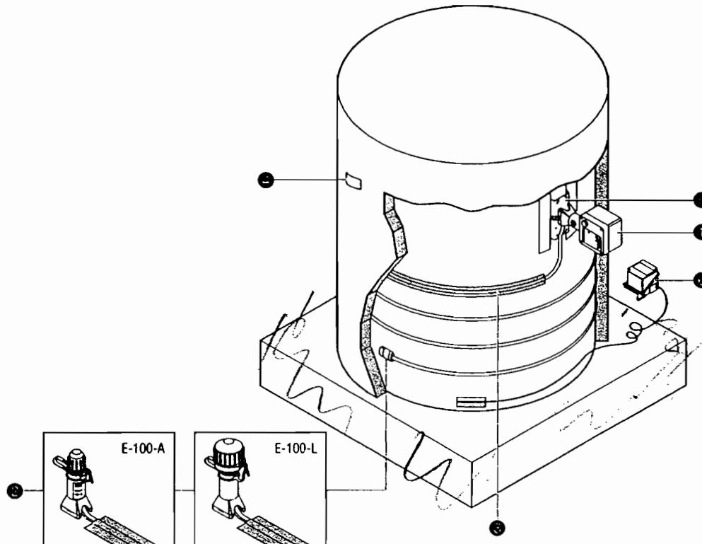
Fig. 9 Tank-tracing system components and accessories
