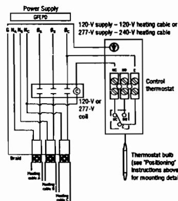
Figure 4. Contactor control
