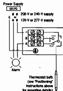
Figure 2. Low-temperature alarm
