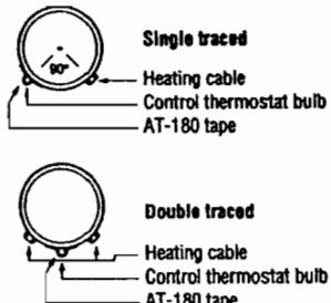
4. Position the bulb in the lower quadrant of the pipe as shown in the diagram to the left. Place the bulb at least three feet from pipe supports, valves, or other heat sinks; protect the capillary from kinks or bends less than 1/2 inch in radius.
