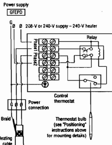
Figure 1. Heat-tracing control
