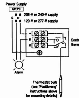
Figure 3. High-temperature alarm
