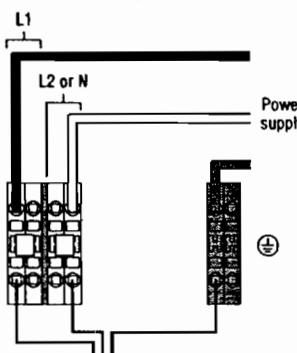
Power connection for two or three heating cables.
