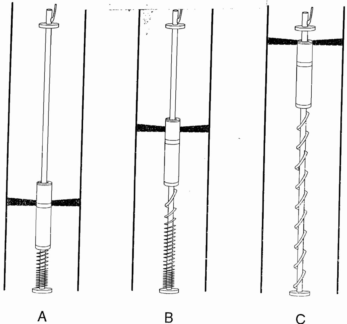
Recommended installation of the SkimRite™ is shown in Figure B.
