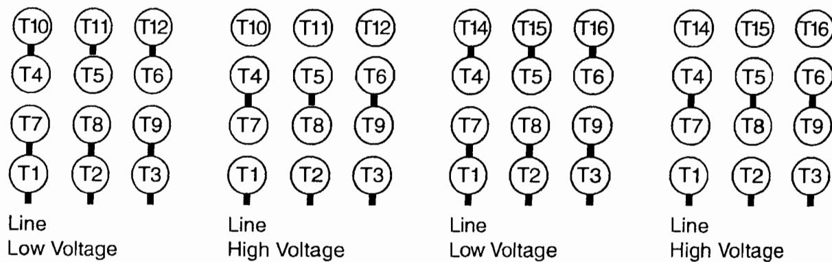
To reverse rotation on any 3-Phase motor, interchange any two external motor line connections to any two line leads.
