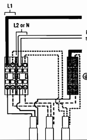
Power connection for two heating cable circuits.
