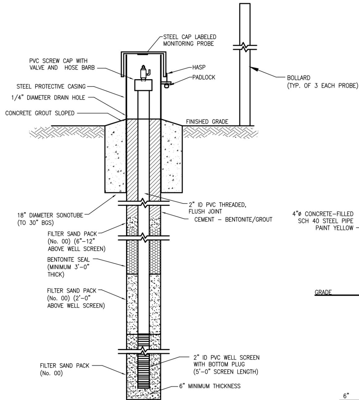
**GAS MONITORING PROBE DETAIL**
