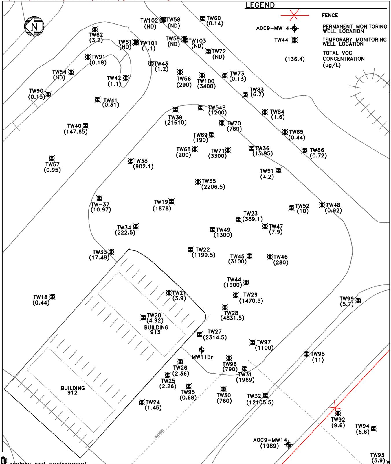
FIGURE 2-2: LOCATION OF TEMPORARY AND PERMANENT MONITORING WELLS AT EXCAVATION SITE
