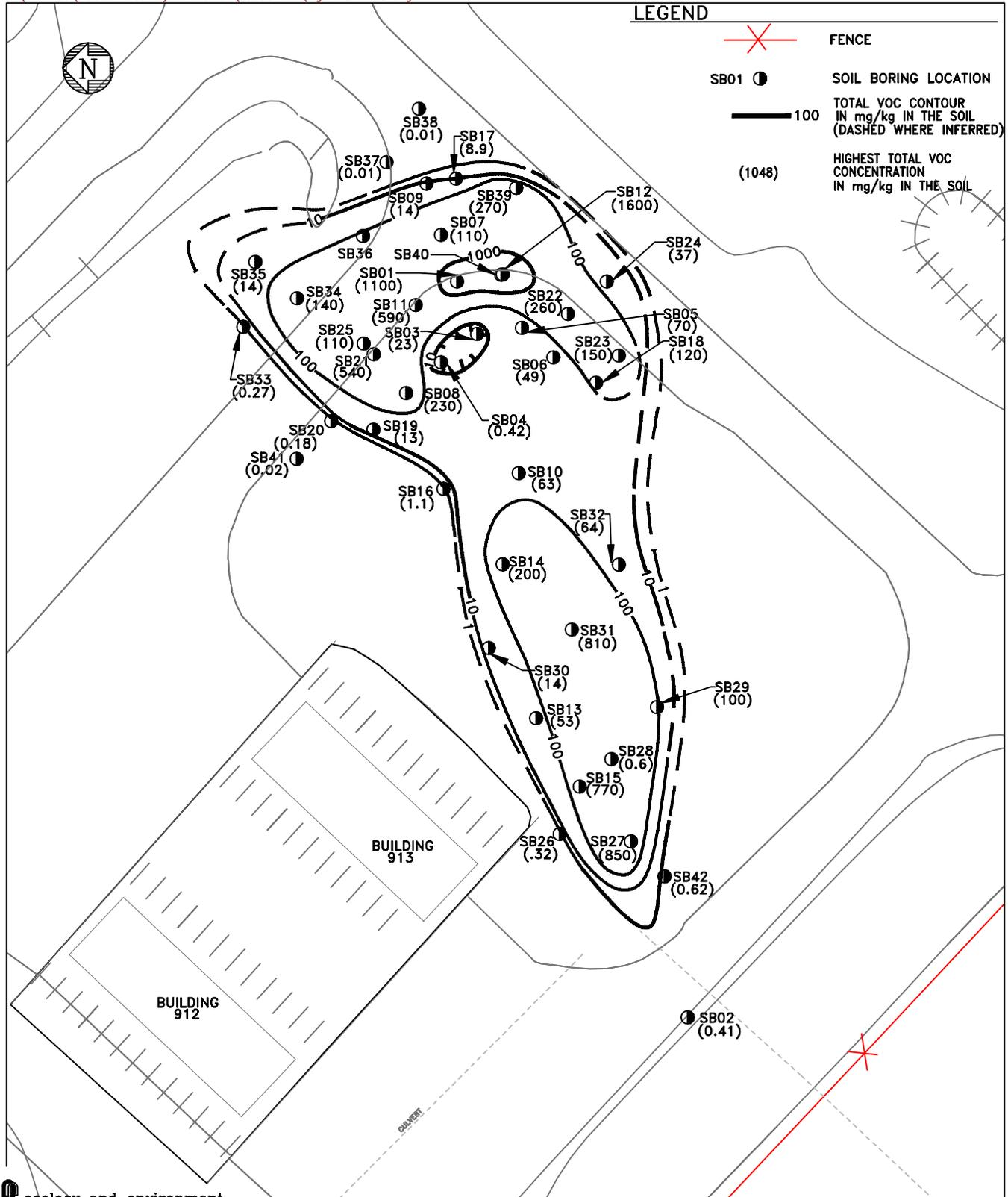
FIGURE 2-3: LOCATION OF SOIL BORINGS AND VOC CONCENTRATIONS AT EXCAVATION SITE
