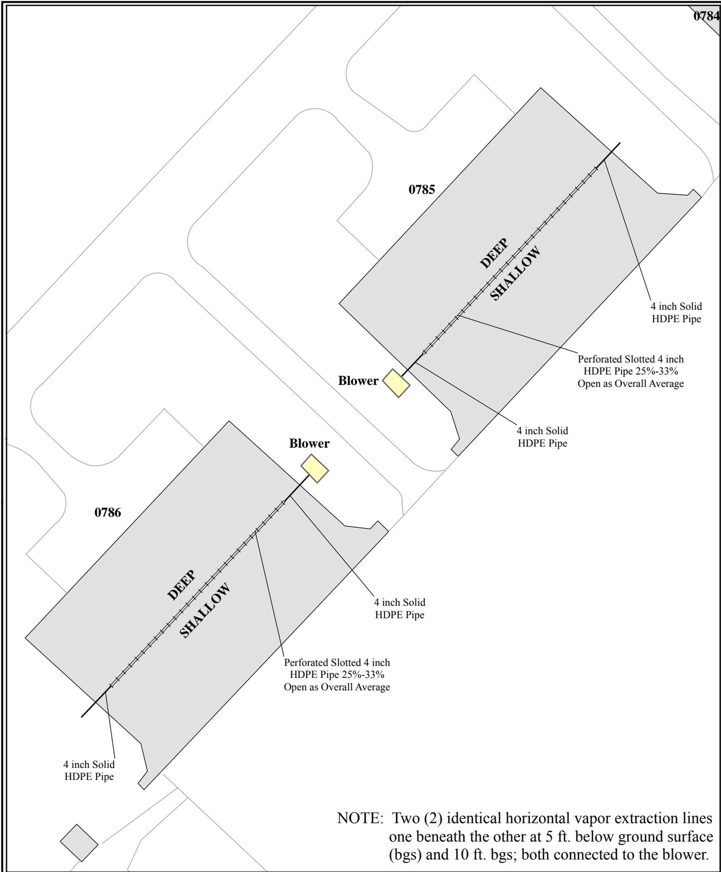
NOTE: Two (2) identical horizontal vapor extraction lines one beneath the other at 5 ft. below ground surface (bgs) and 10 ft. bgs; both connected to the blower.
