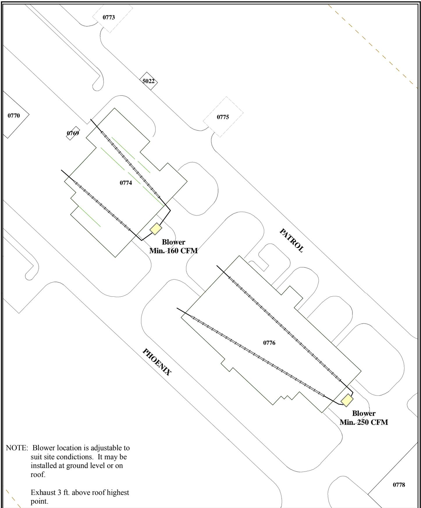
NOTE: Blower location is adjustable to suit site conditions. It may be installed at ground level or on roof.
