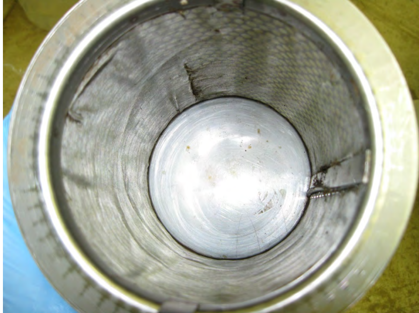
Photo 20 – Close up of basket strainer after cleaning; small tear in the screen is visible at top, center of photo.
