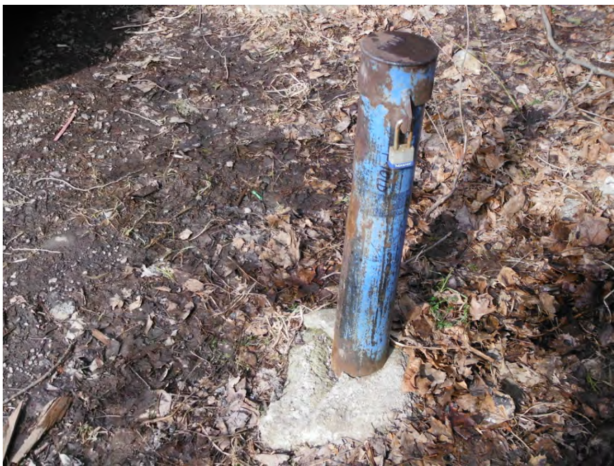
Photo 2: Monitoring Well P-101D cracked concrete, tilted possibly from snow plowing.
