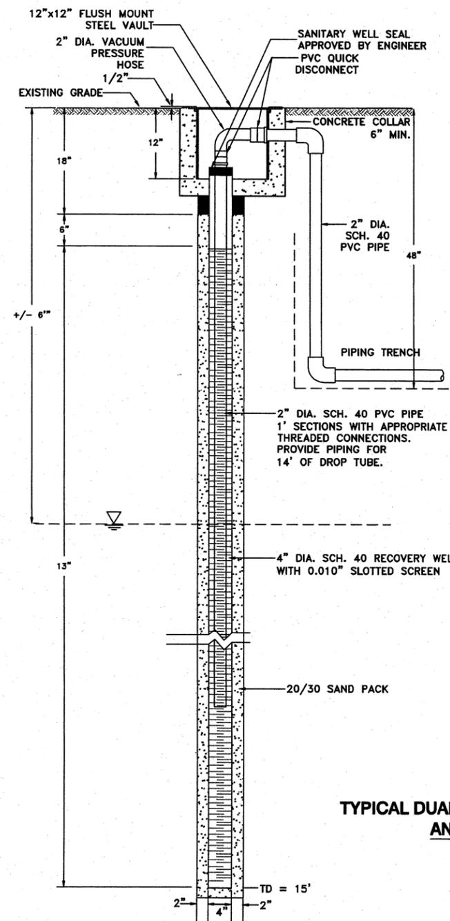
**TYPICAL DUAL-PHASE EXTRACTION WELL AND VAULT DETAIL**
