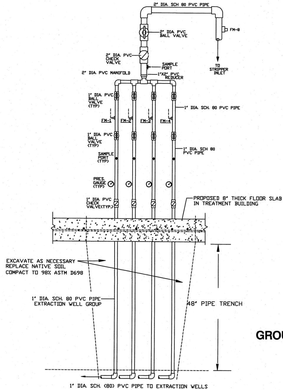
**GROUNDWATER EXTRACTION WELL STUB-UP
