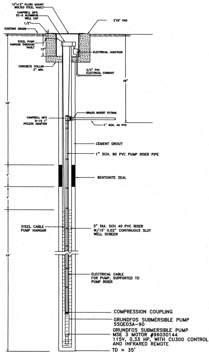
**INTERMEDIATE GROUNDWATER EXTRACTION WELL AND VAULT DETAIL**
