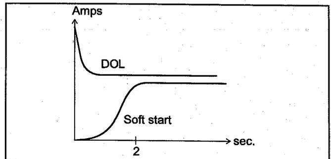
The soft-start will reduce your chance of water hammer, minimizes the risk of wear and prevent overloading of your circuit during start-up.
