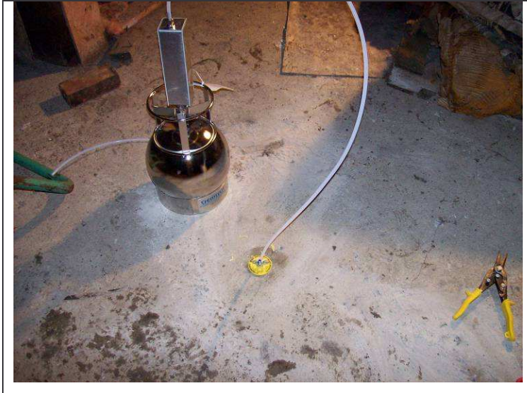
Setup for Sample train at SS-3 subslab vapor location in basement.
