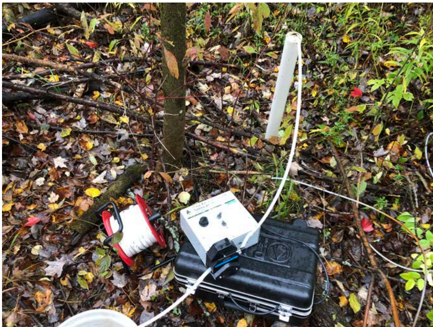
Photo 13 – Well purging activities and field parameter measurements at well TPW-14.
