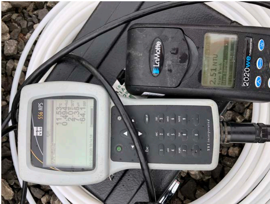
Photo 5 – Final field parameter measurements from well B1231-MW-03.
