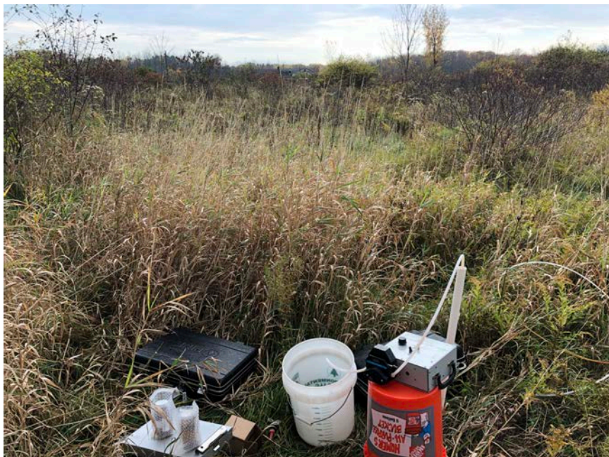
Photo 3 – Well purging activities and field parameter measurements at well B1219-W06.
