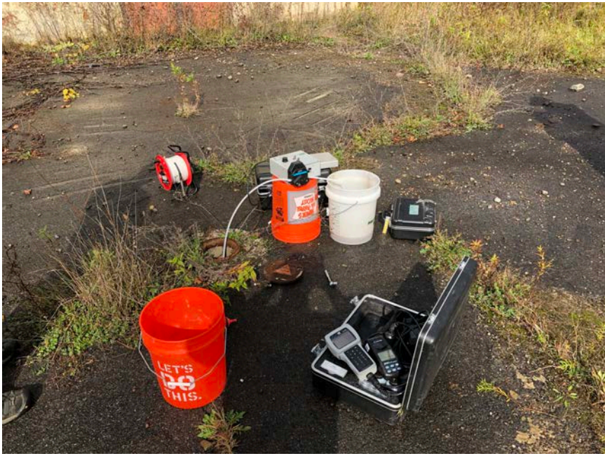
Photo 8 – Well purging activities and field parameter measurements at well MW-1253IR.
