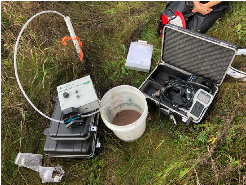
Photo 6 – Well purging activities and field parameter measurements at well B1243-W05.
