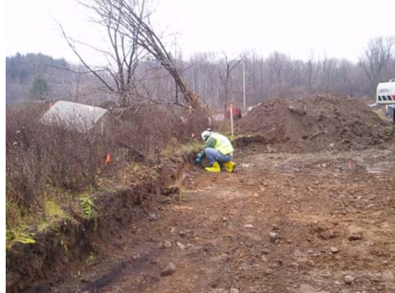
11/26/07 Collection of Sidewall confirmation sample SG-009
