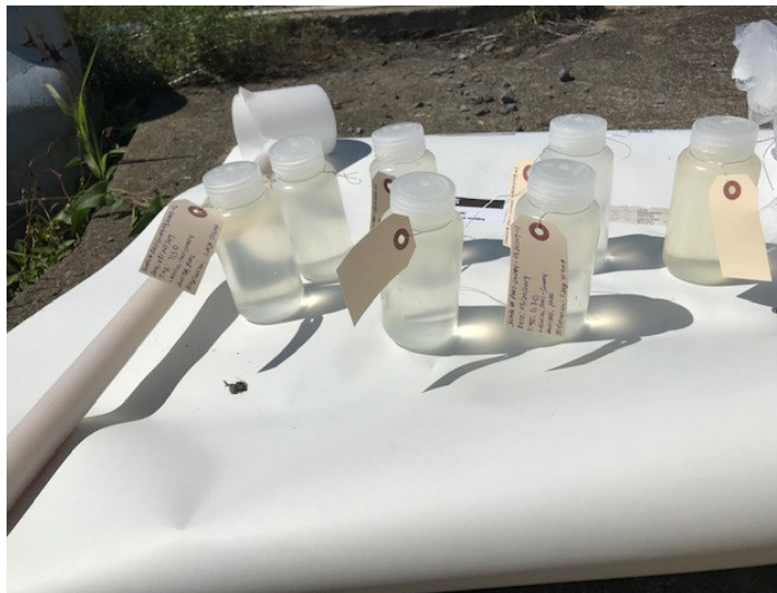
Photograph 7: View of the PFAS sample bottles after they had been collected. Dedicated HDPE, PVC sampling equipment, and sample bottles were placed onto silicone vapor shield to keep equipment and bottles off the ground and free of any PFAS contaminants. Labels were hand written on paper tags to insure that PFAS contamination did not occur from adhesives. Samples were placed into HDPE bags and stored on ice.
