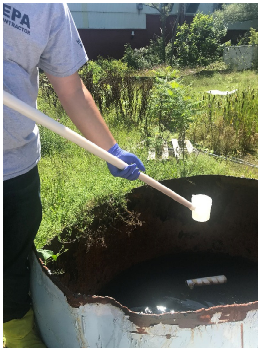
Photograph 8: View of START V team member sampling at SW004. Natural latex booties were worn to add an extra layer of protection, helping to further eliminate PFAS contaminants. The floating material referenced from photograph 6 can also be seen.
