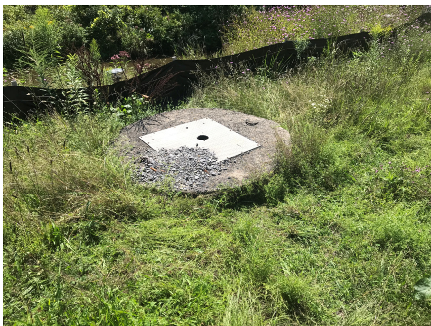
Photograph 4: View of SW002 (Tank 01). A non-weight polyvinyl chloride (PVC) bailer was used to collect the PFAS sample from the approximate 6 inch hole in the top of the tank. After the PFAS sample was collected, START V concluded that a high density polyethylene (HDPE) dipper would fit into the hole. The remaining five samples were collected using that dedicated piece of sampling equipment.
