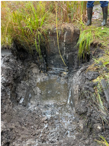
Photo 9: Creosote saturation in test pit TP-1
