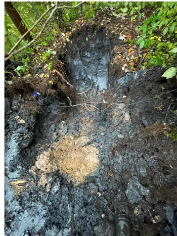
Photo 4: Creosote observed in test pit E11 from approximately 0 to 3 ft bgs.
