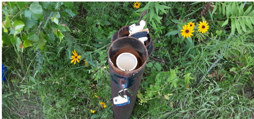
MW-301 Monitoring Well
