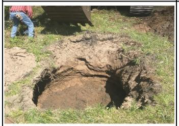
**PHOTOGRAPH 3:** View into the depth of TP-3. Frequent cave-ins occurred due to groundwater saturation and loose, sand and gravel soil.
