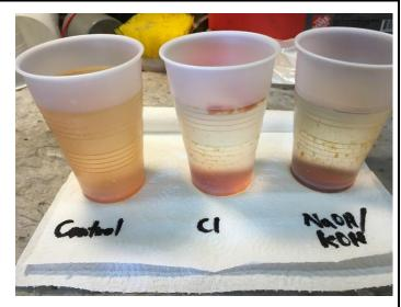
PHOTOGRAPH 18: Photograph of recovery well water iron separation bench testing, taken moments after the test was initiated, with control sample and chlorine solution added and sodium hydroxide/potassium hydroxide solution added samples. Note slow oxidation in the control sample and fast settlement of ferric iron in the treated samples.
