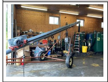
PHOTOGRAPH 25: Inside view of the tube auger loading activated carbon into carbon vessel number 4.
