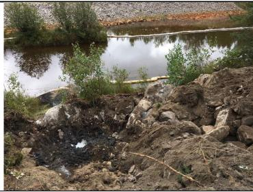
**PHOTOGRAPH 1:** Westerly view of Benson Seep test pit TP-1, depicting gravelly soil with large, angular rock fragments and grey, petroleumstained soil at the bottom of the excavation. The Little River is immediately south (left) of the excavation.
