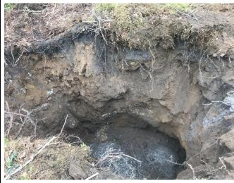
**PHOTOGRAPH 2:** View of TP-4 showing the various soil strata, including miscellaneous fill materials deposited during historical mine operations.
