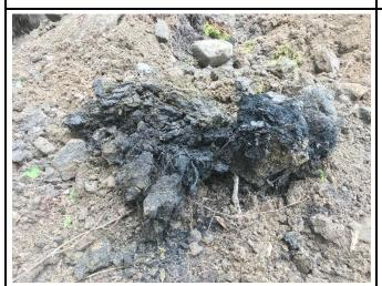
**PHOTOGRAPH 3:** Evidence of "marsh mat" material encountered at approximately 11.5 feet below grade in the TP-5 excavation.
