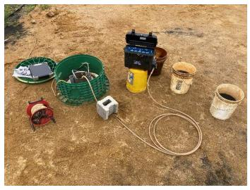
PHOTOGRAPH 22: Peristaltic pump oil recovery operations at RW-6.
