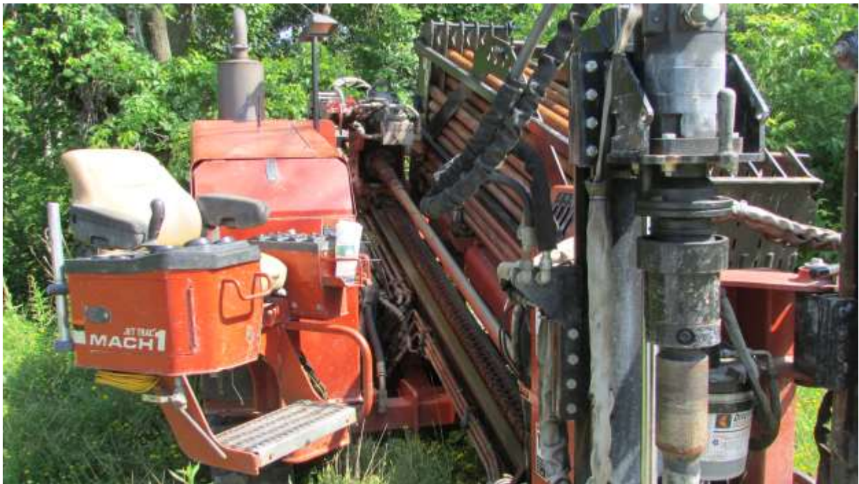
Detail of drill rig showing auto control for adding/removing drill pipe
