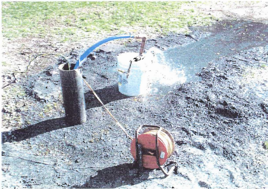
Pumping test at 14 gpm at East Windsor Road; Note: water level indicator and sample port
