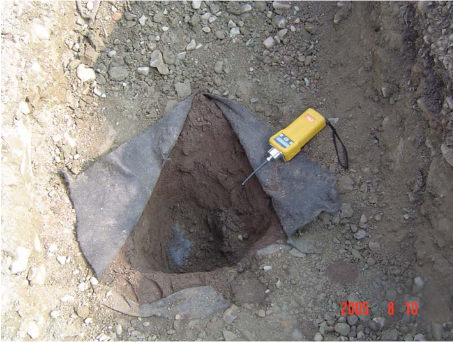
COLE-1 Investigation Location Liner Exposed
