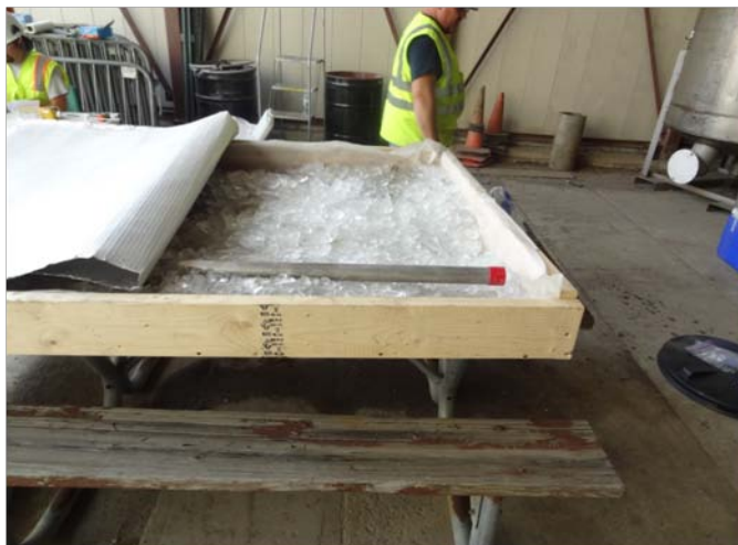
Ice bath cooling for SS Soil Cores
