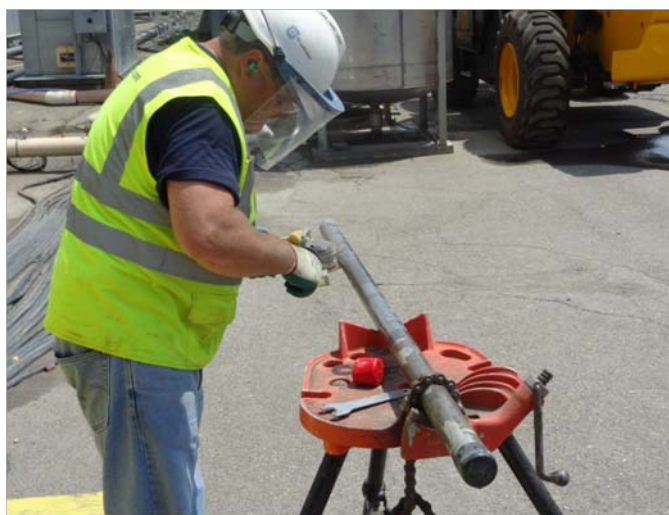
Grinding of SS Macro-cores
