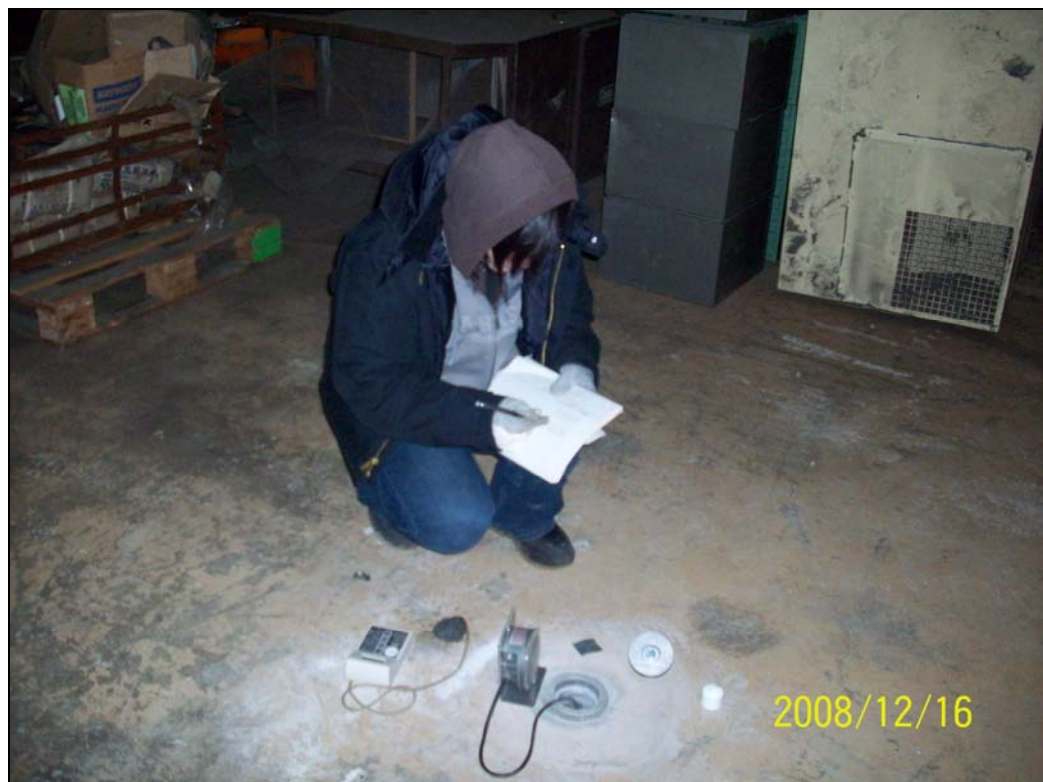
Photo 4 Vacuum pressure monitoring during SVE pilot test, Former Bright Outdoors Site
