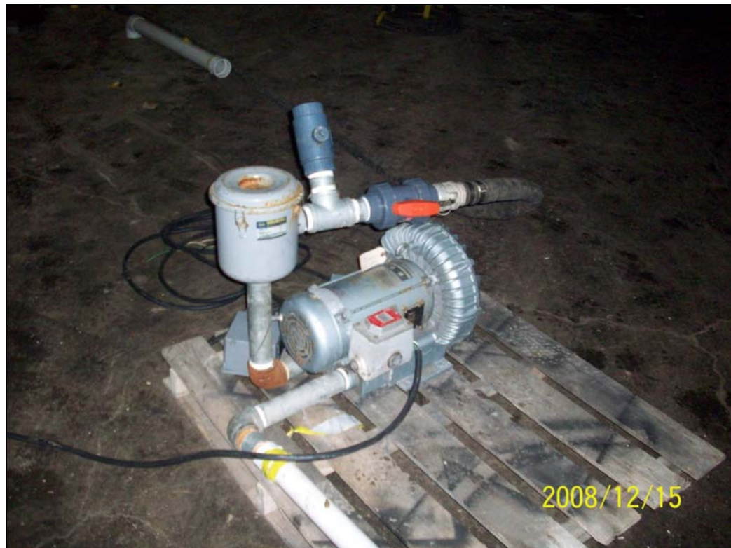
Photo 2 SVE pilot test blower prior to final hookup, Former Bright Outdoors Site
