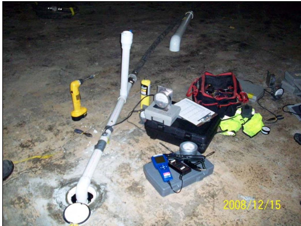
Photo 3 SVE pilot test setup, Former Bright Outdoors Site
