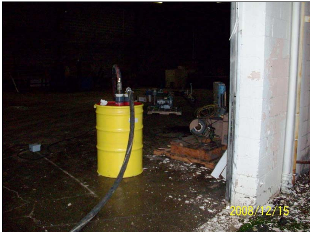
Photo 6 Vapor-phase activated carbon discharge treatment during SVE pilot test, Former Bright Outdoors Site
