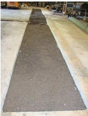
Figure 1: View of stone placement in trench (Looking North AM)
