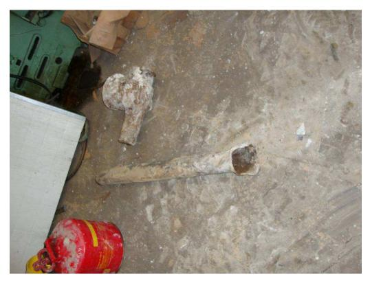
Figure 2: View of cast iron drainage pipe that broke off during concrete removal (Looking East AM)
