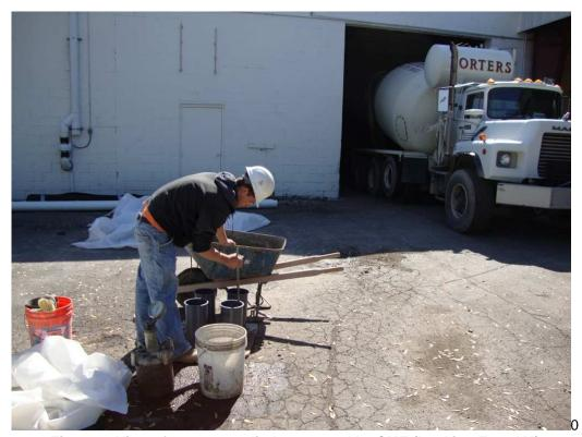
Figure 6: View of concrete cylinders poured by CME (Looking East AM)
