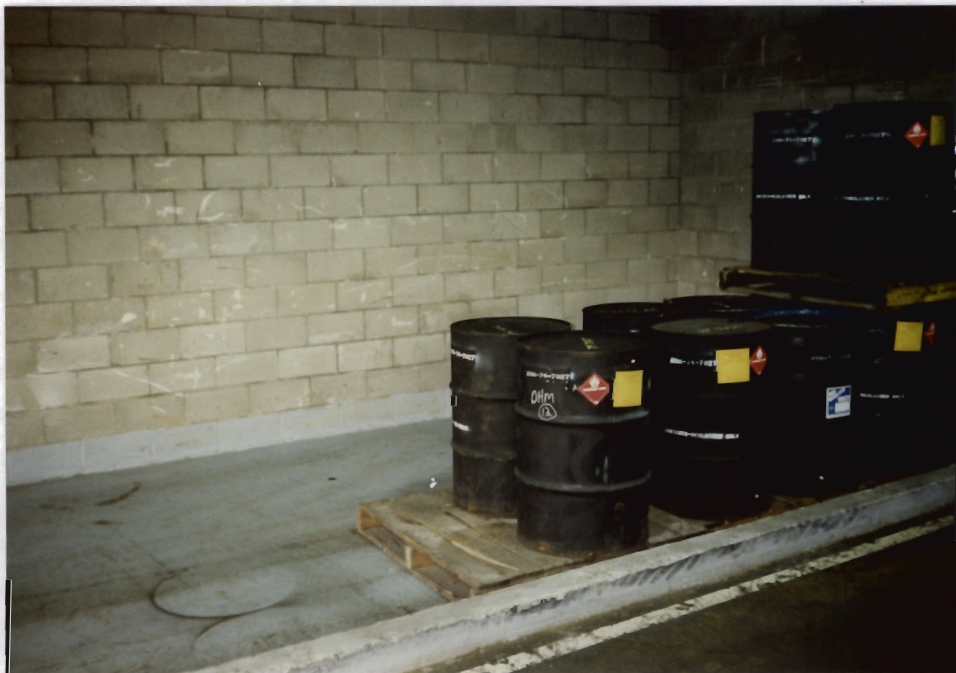
2. View of additional drum storage for flammable wastes at the Hazardous Waste Container Storage and Staging Area (SWMU 1).
