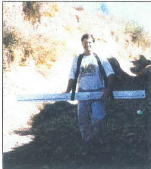
Figure A-1. Photograph of the Geophex Electromagnetic (GEM-2) instrument during a site characterization study.
