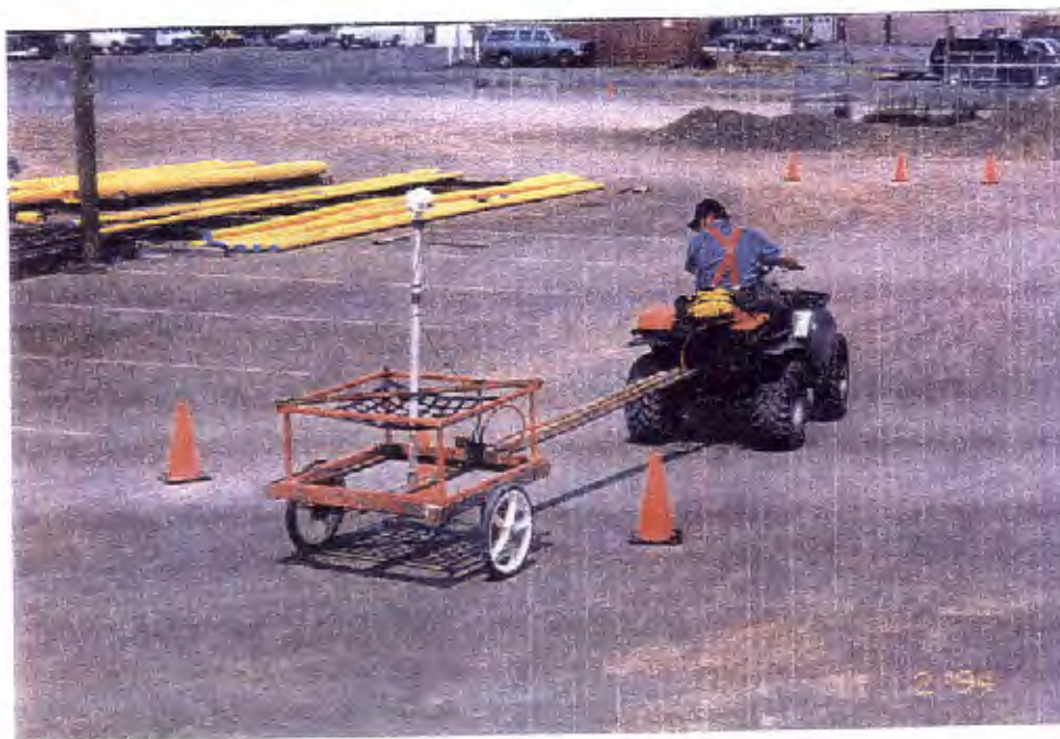
Figure 1: The EM61 and DGPS Survey Setup
