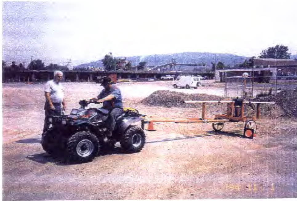
Figure 2: The EM31 and DGPS Survey Set Up
