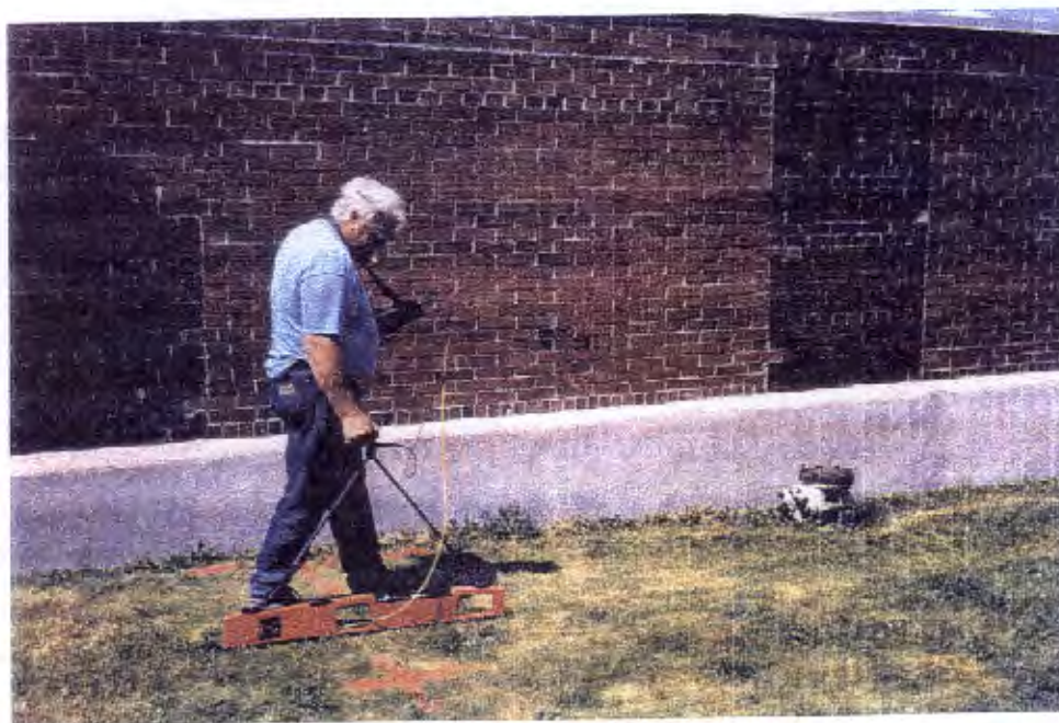
Figure 3: The EM38 Survey Set Up
