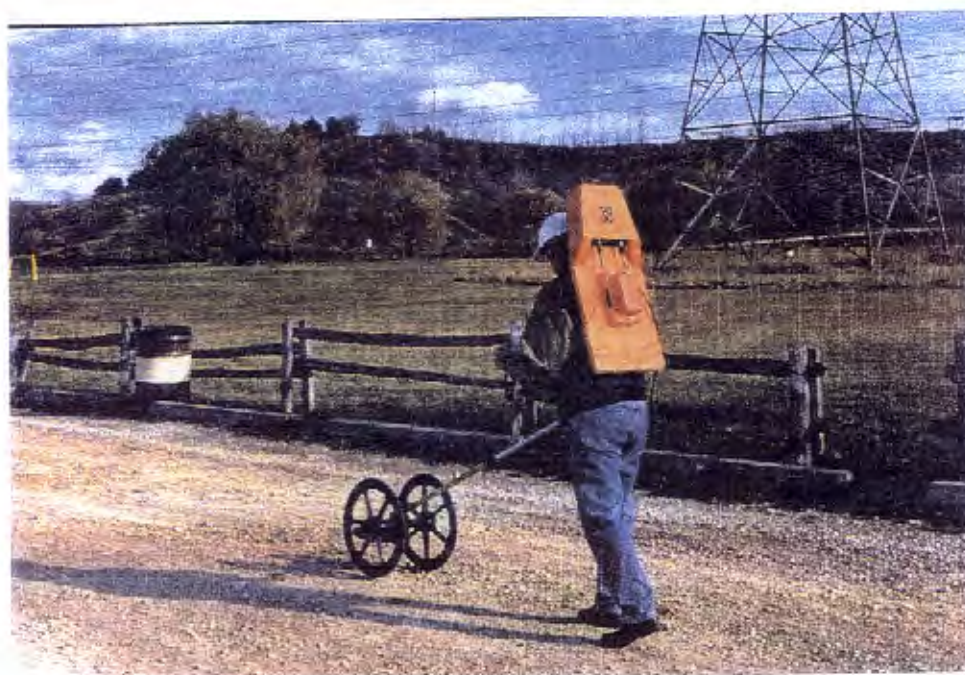
Figure 4: The EM61-HH Survey Set Up
