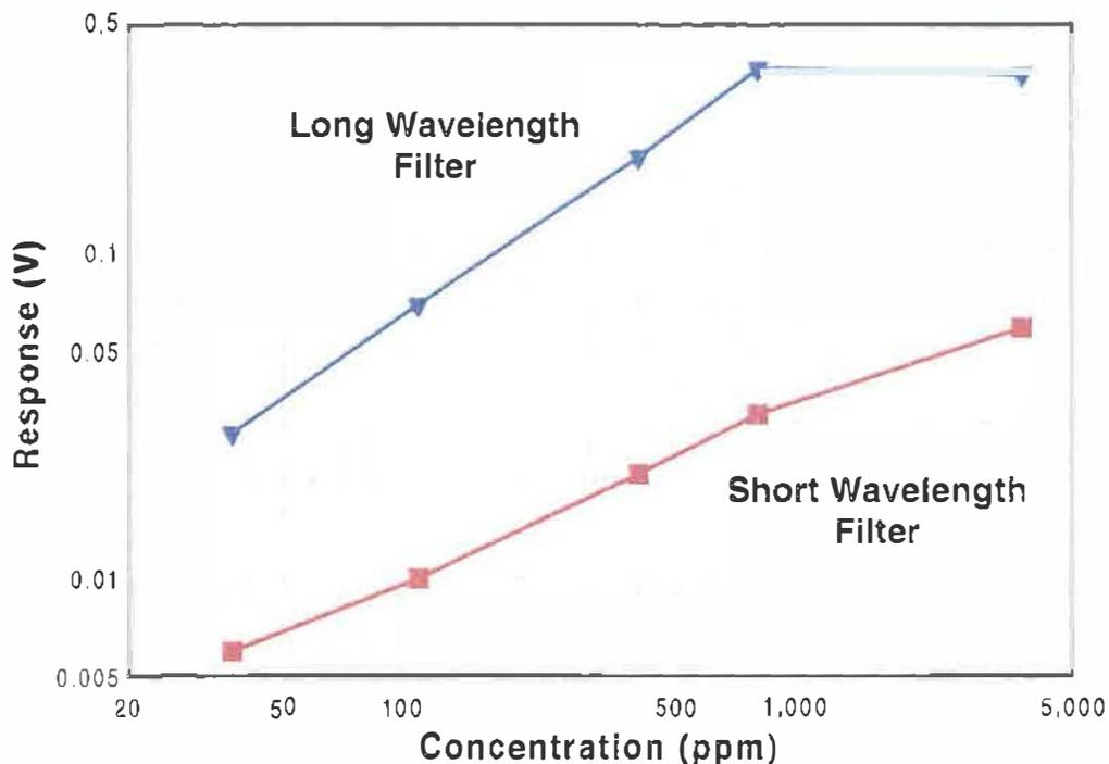
**Figure 1. Response of the ARA Fuel Fluorescence Detector to product from the Court Street MGP site in clean sand using two different detection wavelength ranges.**
