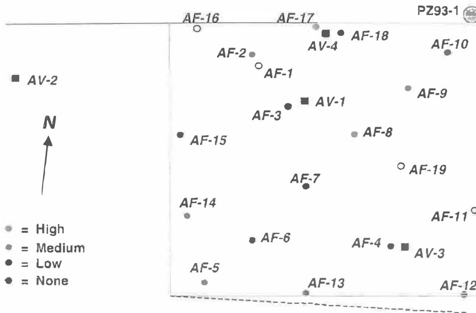
**Figure 2. Map of CPT deployment locations in the demonstration zone and peak contamination levels measured with the FFD.**
