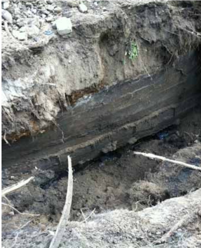
Photo #7 (2011.09.15):CTP-5. Gas holder #1 wall runs along length of test pit. Wall along east side of test pit. Stained soil beneath holder foundation.
