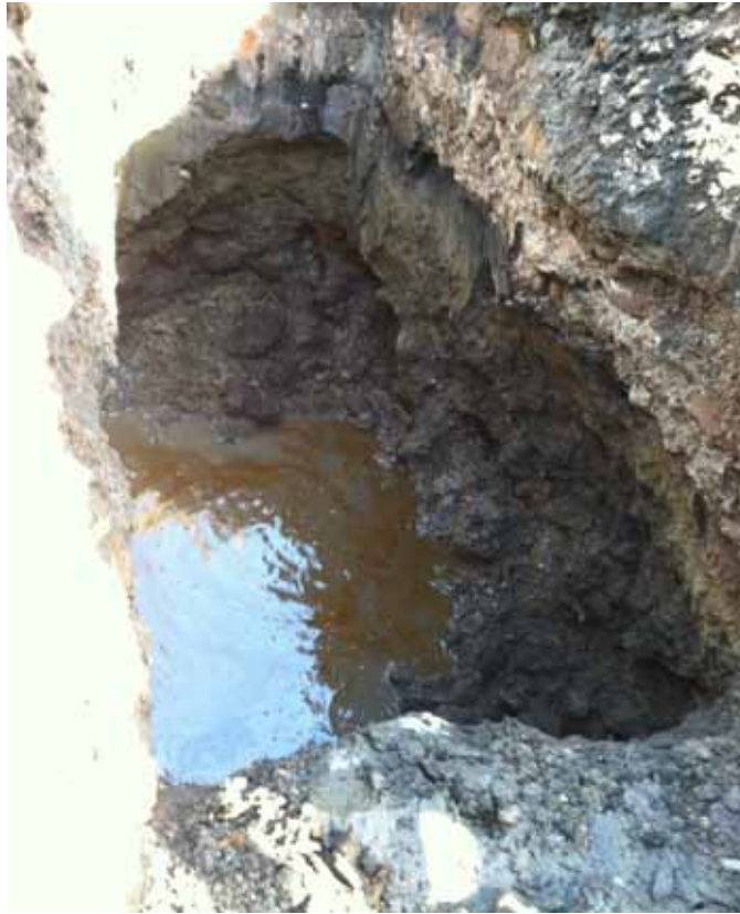
Photo #13 (2011.09.16): CTP-8. Looking south. NAPL from 6 to 8 ft bgs.
