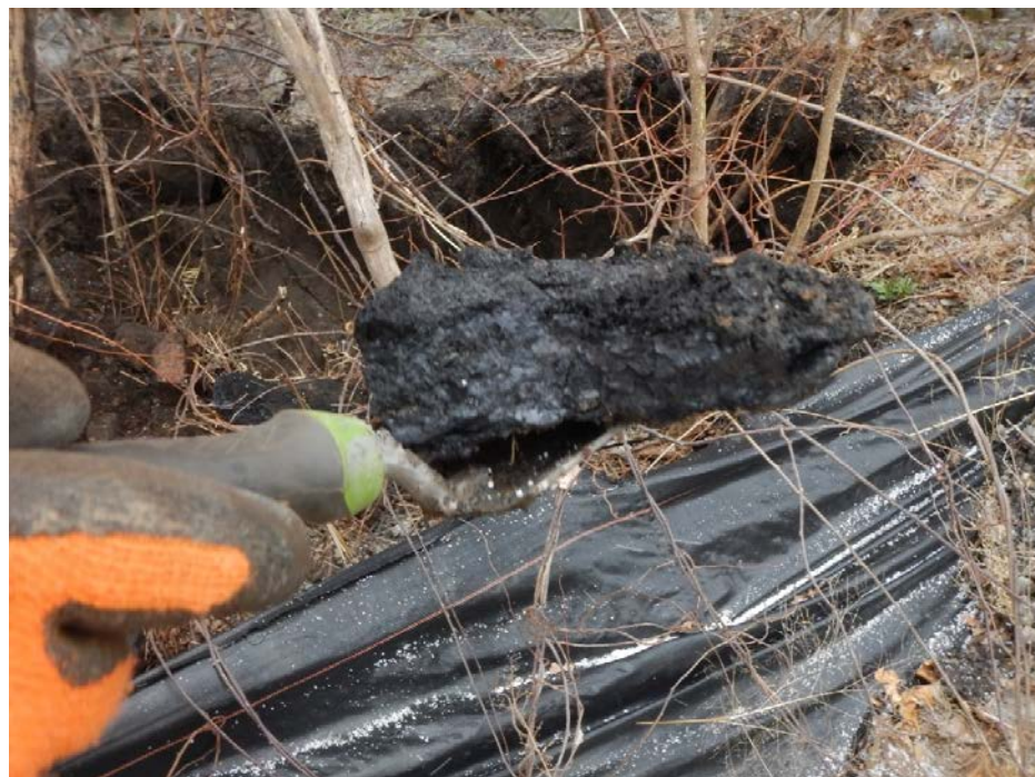
TP-BANK-5 Picture of broken piece of solid coal tar
