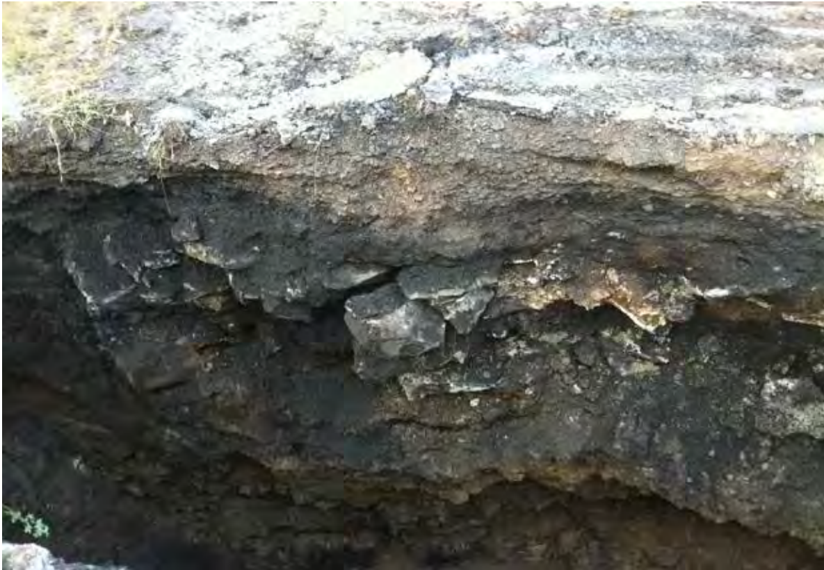
Photo #1 (2010.09.12): MTP-1A. Stone wall located at 1.5' bgs.
