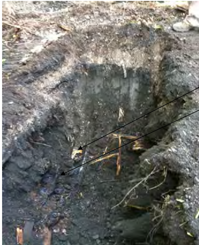
Photo #16 (2010.09.13): MTP-4A. Just east of red brick/wood timbers at NAPL coated soil (3 – 5' bgs).
