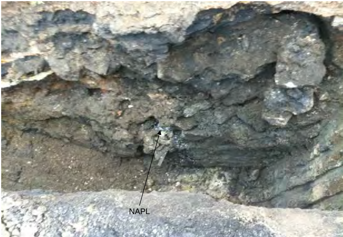
Photo #20 (2010.09.20): MTP-5. NAPL coated area 7 – 9' bgs on south stone wall.
