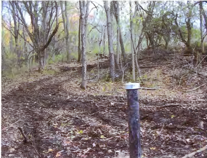
Photograph 7. Downgradient monitoring well MW-4 located in the drainage area near the northwest portion of the sludge disposal area. View facing the northeast with well head in foreground and path used to access drainage area from the sludge disposal area shown in background.
