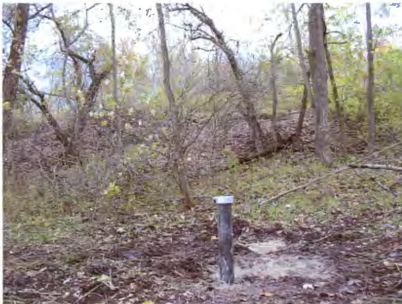
Photograph 8. Downgradient monitoring well MW-3 located in the drainage area near the southwest portion of the sludge disposal area. View with monitoring well in foreground and sludge embankment in background.
