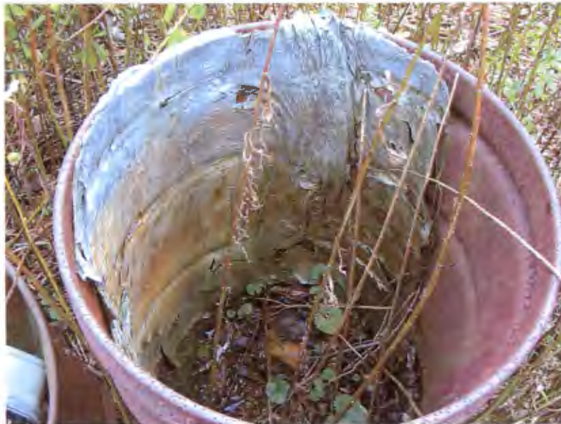
Photograph 7. Drum (south) containing silver colored material on inside wall of drum. Material appeared to have been melted. Vegetation observed in drum, bottom of drum missing.
