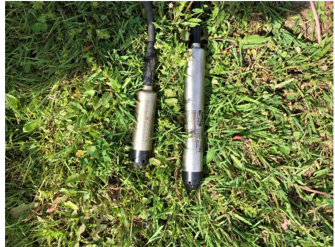
Old (left) and replacement RW-1 pressure transducer.
